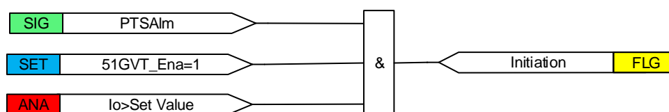
Figure 3.4-5 The Initiation logic diagram for 51GVT
