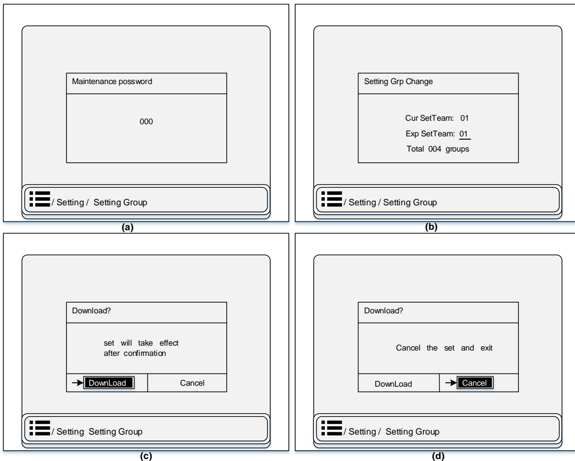
Figure 7.3-22 Procedure Diagram of Group Setting Change
