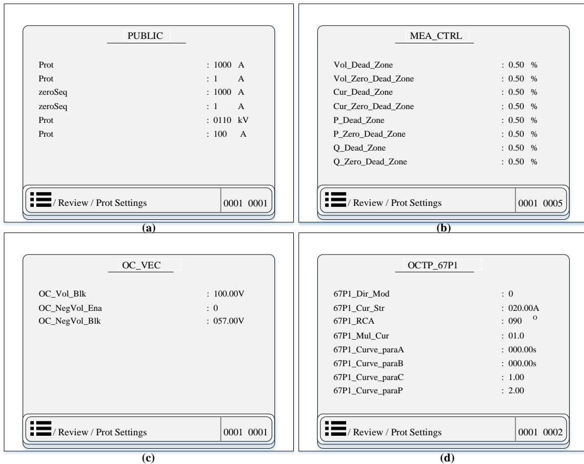
Figure 7.3.6 Overview Diagram of Prot Setting (a) Public Setting (b) Measurement Control Setting (c) Overcurrent Protection Setting (d) Phase Overcurrent Protection Setting of Stage 1
